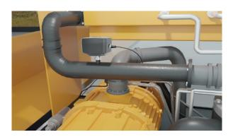
Sensor Installation outside of the compressor
