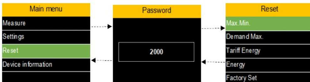
Press or to switch the display of the interface. Press **OK** Key to enter parameter configuration.
