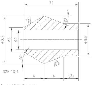
You need to use the cone In the picture above on a hole of about Ø6 - Ø7 with sharp edge, place on the same axis of the transducers hole, i.e. of the fillet
