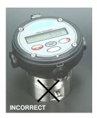
The meter will operate in the alternative orientation, however, it is likely its life & performance will be reduced as a result of the gravity pull on the rotors.
