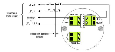
**2.3.5 Bi-directional flow** Combining the Quadrature feature and model PD1 pulse discriminator module produces forward & reverse outputs both of which may be integrated to provide a "net" reading. The RT12 flow rate totaliser will take both output & will perform the "net" flow function.
