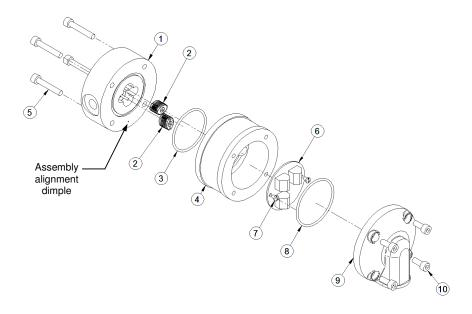
**4.5 Re-assembly of meter** (refer Exploded View) When replacing the rotors be <u>very sure</u> to have the rounded tooth ends at the bottom of the measuring chamber otherwise the rotors will be severely damaged as the meter cap (4) is fastened into place.
