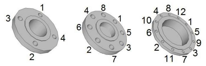
If the bolts are tightened too much during the installation of pipework components, deformation of the sealing surface may occur. In consequence, the torque values indicated in the table are used as a guidance for tightening the screws and bolts.
