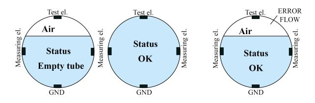
2) incorrect installation (placing the unit diagonally, Empty test - ON)
