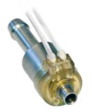
Gas injection **Type VA 204-507 Assembly with 3-way Spider®-Valve, size 15 mm, direct actuated, NC** Orifice (DN): 1.5 mm Pressure: 0...6 bar Medium: Liquid gas Valve body: Brass
