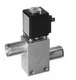
Emission control **Type VA 204-519 2-way Spider®-Valve, size 15 mm, direct actuated, NC** Orifice (DN): 0.6 mm Pressure: 1...6 mbar Medium: AdBlue® Valve body: Stainless steel
