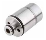
A/C control **Type MA 203-009 2-way solenoid valve, direct actuated, NC** Orifice (DN): 26 mm Pressure: 0...0.1 bar Medium: Air Valve body: Aluminium
