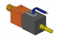
Heating system **Type MA 202-007 2-way solenoid valve, direct actuated, NC** Orifice (DN): 3.5 mm Pressure: 0...1 bar Medium: Gasoline, diesel Valve body: Aluminium
