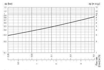
Reference conditions: upstream pressure = 8 bar downstream pressure = 3 bar
